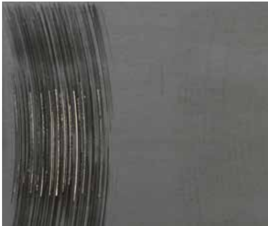
Anti-burnishing and Abrasion Resistance Dead Flat Water-Based Polyacrylic Coating. Comparison of a polyacrylic water-based coating matted with silica vs a 90:10 blend of Silica:ACumist A-6.
